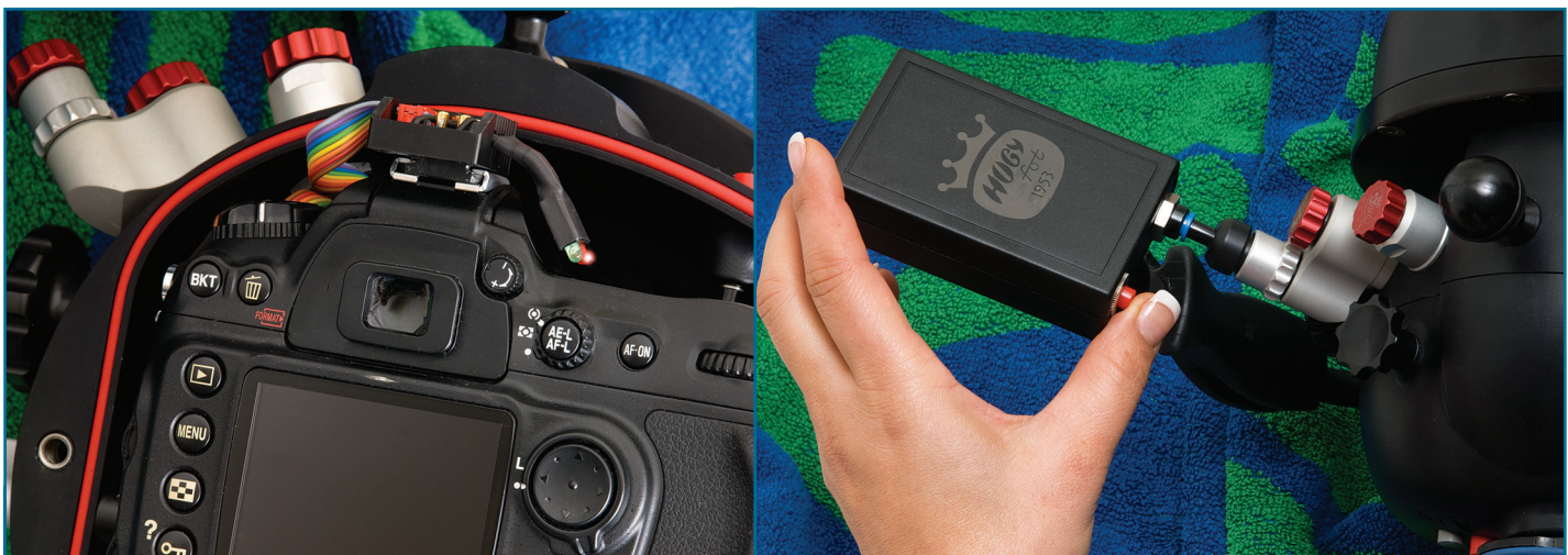
From left: The Hugyfot housing incorporates a pressure-sensor; inserting the mini vacuum pump.
