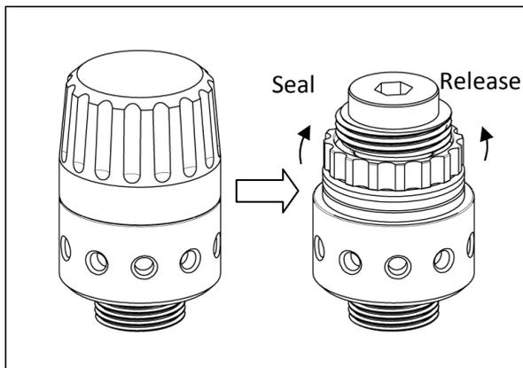
1. Remove the vacuum valve cap.
