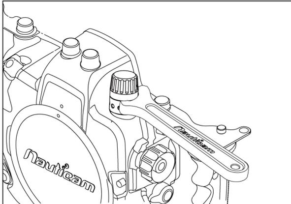
1. Remove the plug of the M14/M16 accessory port (or other accessory bulkhead) from the housing.
