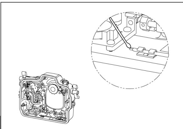
2. Test the moisture alarm by contacting the two wires near the bottom of the housing with a damped cotton bud; the alarm should start giving out a repeating “beep” sound along with a flashing red light. The “beep” sound and the light should keep on going for 5 seconds after the removal of the damped cotton bud .
