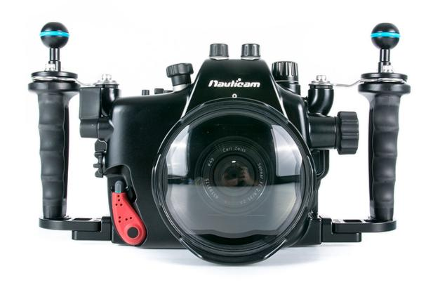
Of course, the sort of quality and robustness that has become synonymous with the Nauticam name is present with this housing as well. Milled from solid aluminum, the housing is depth rated at 100m and built to last. Exceptional care is taken to reduce any possibility of galvanic corrosion, and the housing is hard anodized to stay looking great after years of use.
