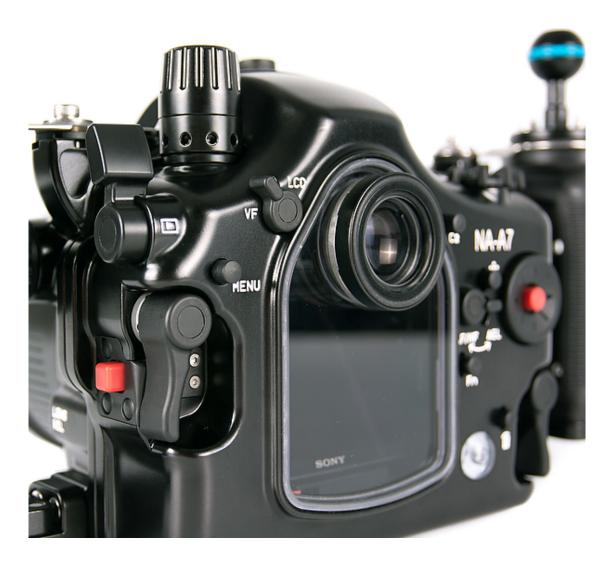
The patent pending EVF/LCD switch allows a quick way to alternate between using the large bright LCD display or the high resolution electronic viewfinder (EVF). The housing ships with a standard .66x viewfinder for the EVF, which is easily swapped out for either of the two Nauticam enhanced viewfinders.
