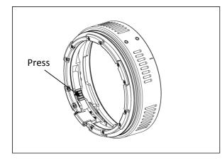
1. Press the RED bar to unlock the locking device of the extension ring.
