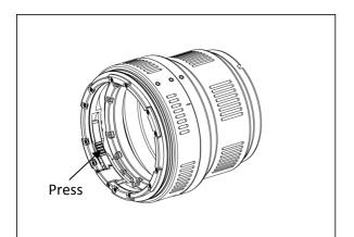
6. To unlock, press the RED bar to release the locking device and reverse the above procedures.
