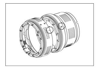
2. Align the "I" mark on the extension ring with the WHITE dot on the port.
